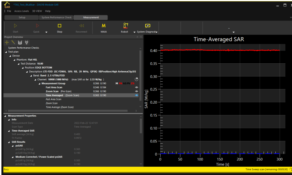
Figure 1.7: Optional single-point SAR measurements confirming that the output power of the phone is stable - the DPC-ETA algorithm is not controlling it
